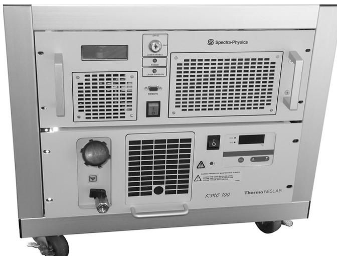
**Figure 5-7: The power supply and chiller on the rack.**
