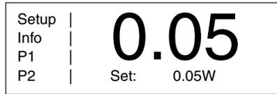
To change the power setpoint, either press one of the preset power setpoint keys (P1 or P2) to move directly to a power previously set in the Setup menu, or use the up/down buttons to set a new value. Note that when the up/down buttons are held in, the setpoint numerical update pauses from time to time. This is normal.
