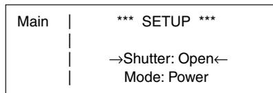
To access this menu from the Main menu, use the two lower left buttons to scroll the menu up and down. The selected item is the one between the horizontal arrows (the example screen above shows the shutter status, which can be set to open or close). To change the value for the selected item, use the up/down buttons to the right of the screen.
